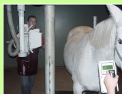
Figure 3. Measuring the scatter dose with a dosimeter.
